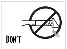
Allow crushed or clogged ducts and vent.
